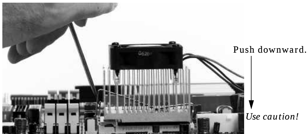
Figure 15. Pushing the Heatsink Clip Down
